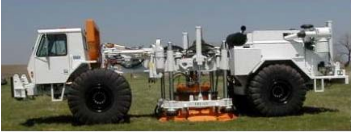
Figure 3 "T-Rex" Tri-axial Vibrator was used as the source of energy for deeper shear wave velocity profiling.
